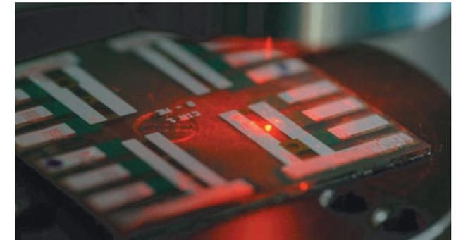
Transparent perovskite light emitting diodes on sapphire substrate with scaled emission area for injection of ultrahigh current densities
