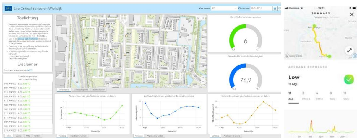
**Figure 8: Left: map visualization of a fixed sensor network in Wielwijk, Dordrecht (NL) with temporal variation of the past hours (left), and right: daily exposure quantified by wearable sensor in Antwerp on a map and temporal graph**
