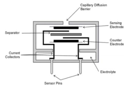
**Figure 3: Working principle of particle sensors (left) and electrochemical  $\text{NO}_2$  sensors (right)**
