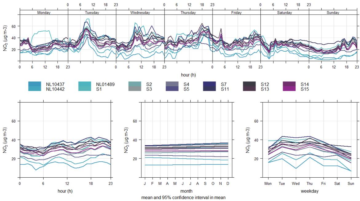
**Figure 9: Time variation graphs (R openair package) of NO<sub>2</sub> data collected from a supplementary sensor network in Dordrecht (S1-S15) and 3 nearest reference monitoring locations (NL10437, NL01489, NL10442)**
