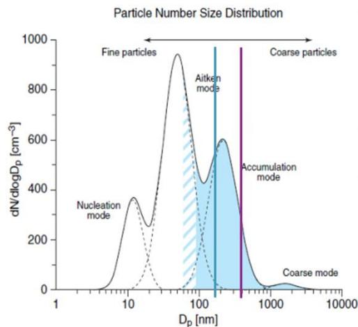
**Figure 4: Lower detection limit of low-cost sensors (purple), compared to equivalent instrumentation (blue), visualized on a typical particle number size distribution (particle counts (#  $\text{cm}^{-3}$ ) vs particle diameter ( $D_p$ ))**
