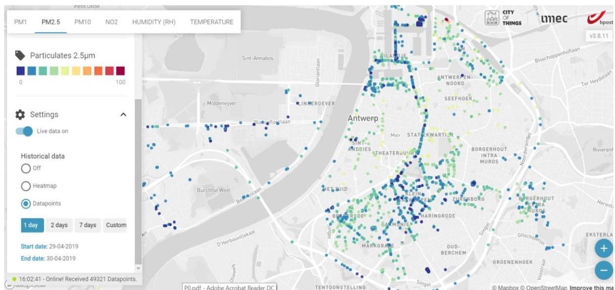
**Figure 13: Mapping Air Quality (MAQY) dashboard visualizing mobile air quality measurements ( $PM_1$ ,  $PM_{2.5}$ ,  $PM_{10}$  and  $NO_2$ ) collected during one day (29/4/2019) by postal vans in Antwerp (BE)**
