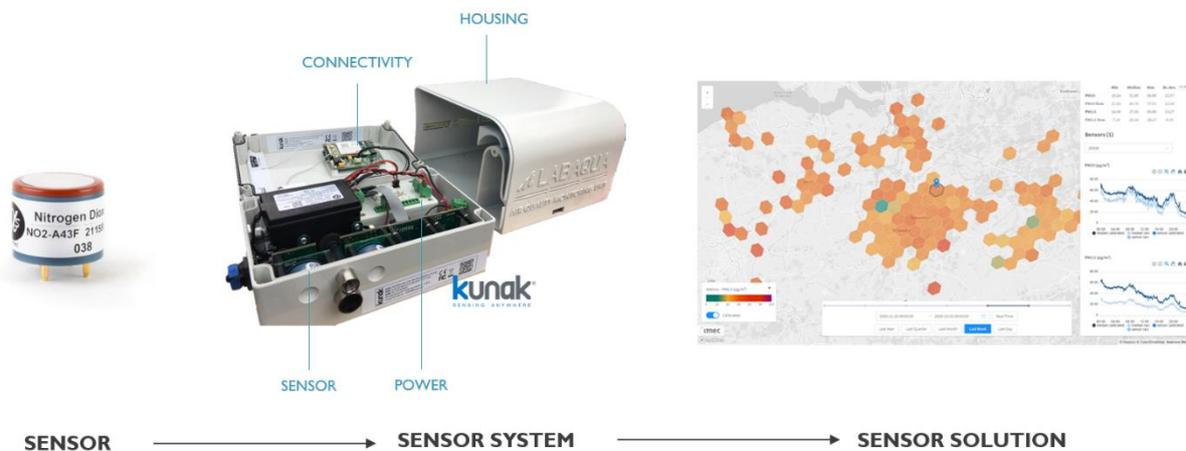
Figure 2: Difference between sensor, sensor system and sensor solution
