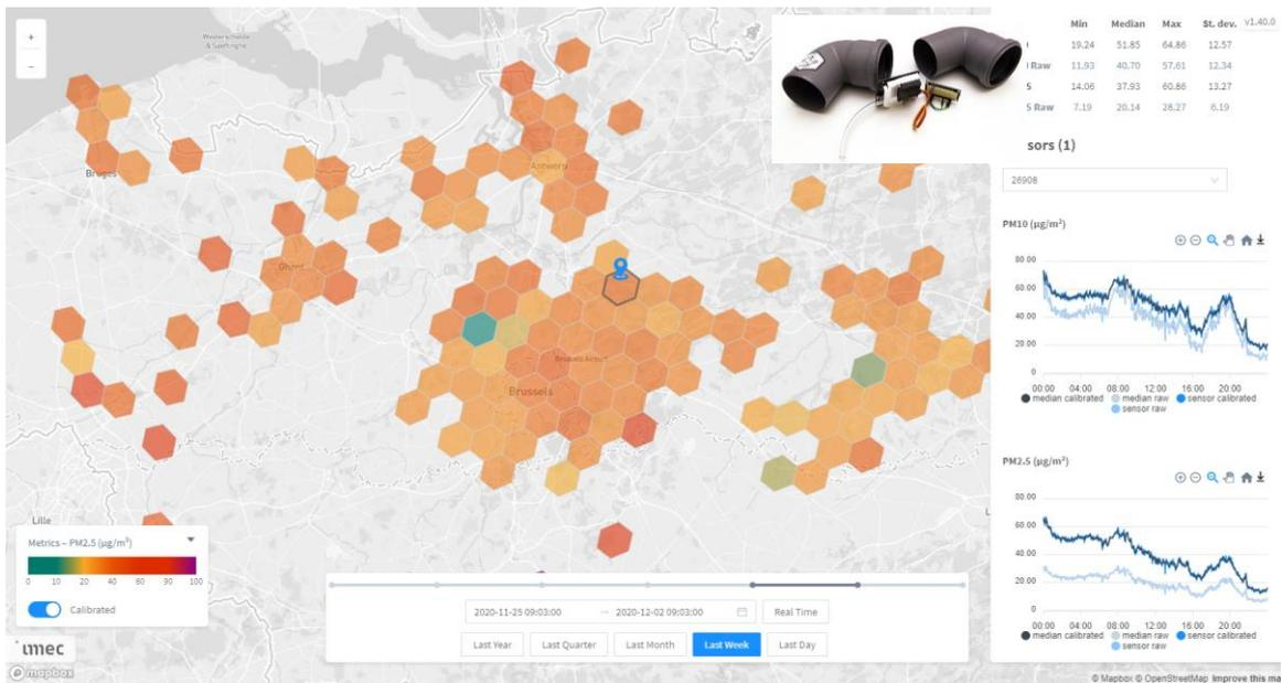
**Figure 7: Visualization dashboard showing IMEC-NL's real-time calibrated sensor data from openly available PM sensors (<https://sensor.community/nl/>)**
