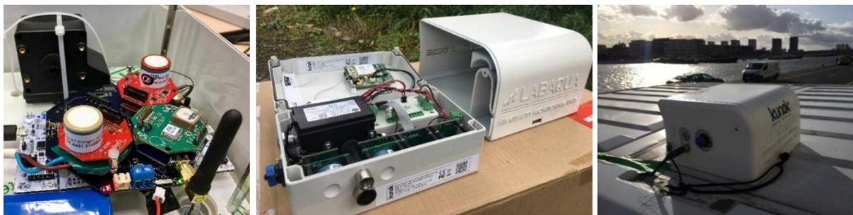
**Figure 5: IMEC OCTA platform including Alphasense PM, NO<sub>2</sub> and O<sub>3</sub> sensor and LoRa antenna (left), mobile Kunak sensor hardware and dedicated housing for optimized flow conditions (middle) and picture of a deployed Kunak sensor on the roof of a Bpost van (right)**
