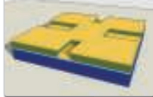
Electrode metallization by sputtering or evaporation
