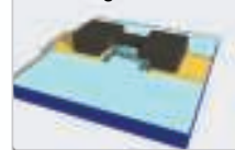
Mask and ribbon are thinned by differential fib milling (low kV)
