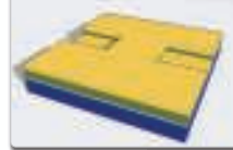
Electrode metallization by sputtering or evaporation
